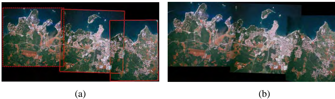
Figure 8: Geo-referenced based image mosaicking example (a) input images, (b) output mosaiced image [56]
